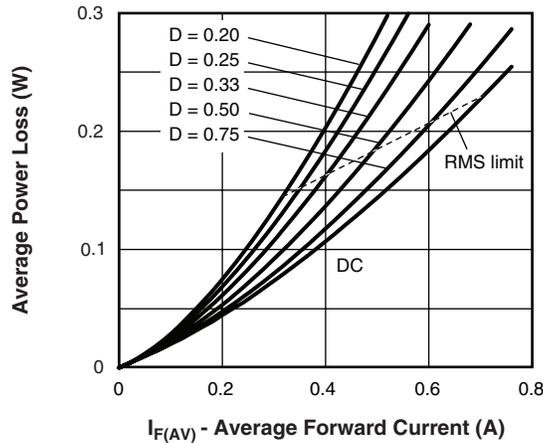
Fig. 5 - Forward Power Loss Characteristics (Per Leg)
