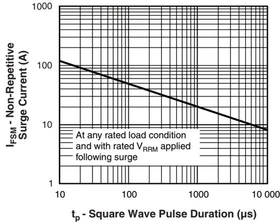
Fig. 6 - Maximum Non-Repetitive Surge Current (Per Leg)
